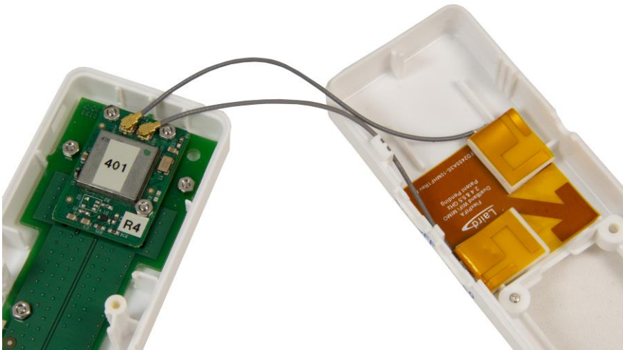
Figure 2: Typical placement of FlexPIFA MIMO within a plastic electronic package
