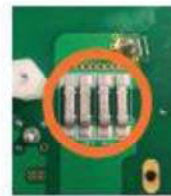
Remove jumpers and add a cable for inductor current measurement
