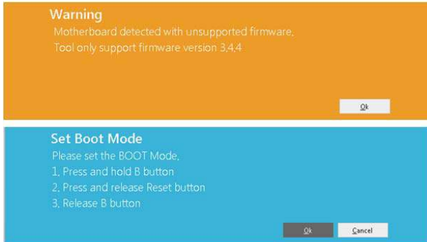
Figure 7. Updating the EVAL-ADPDM3Z Firmware
