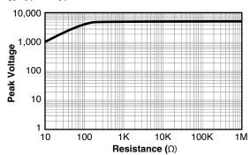
TRHE are tested in accordance with IEC61000-4-5, waveform  $1.2/50\mu$ s, 10 pulses applied. Limit of acceptance is a shift in resistance of less then 1% from the initial value.
