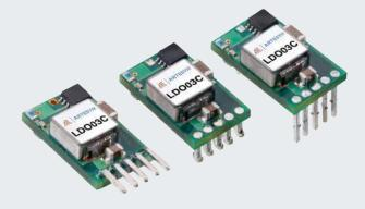
Advanced Energy's Artesyn LDO03C series non-isolated DC-DC converter is designed for cost- and space-sensitive applications. It has a wide 3–13.8 Vdc input range and offers a 0.59–5.1 Vdc adjustable output that accommodates a wide variety of silicon power needs. Capable of delivering up to 3 amps, the converter has a typical efficiency of 90%. A remote enable facility is provided as standard and remote 'power good' indication is available as an option.
