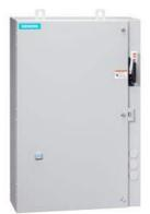
Non-reversing motor starter, Size 3, Three phase full voltage, Solid-state overload relay, OLR amp range 25-100A, 240V 50Hz / 277V 60Hz coil, Combination type, 100A fusible disconnect, 100A/600V fuse clip, Enclosure NEMA type 4/12, Water/dust tight for outdoors, Extra-wide enclosure
