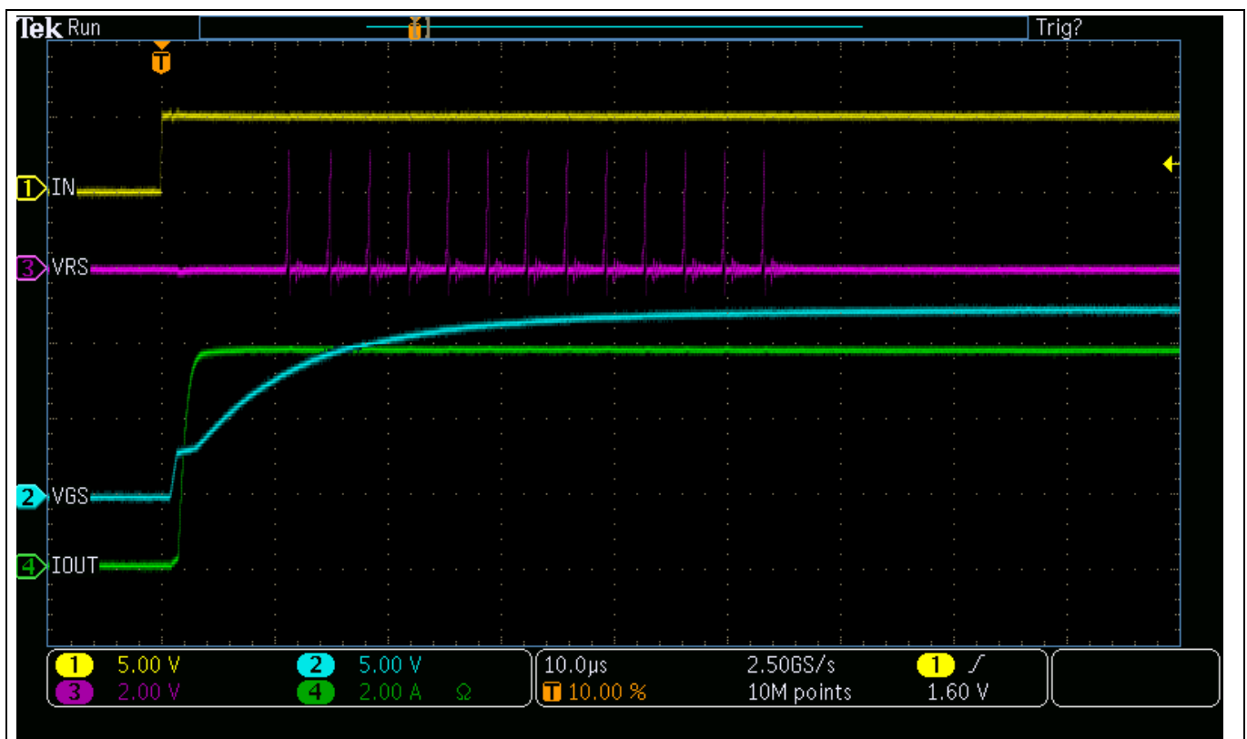
Figure 4 Waveforms from OFF to ON mode [Yellow V_{IN} ; Blue V_{GS(AUIR3241S)} ; Purple V_{RS} ; Green I_{OUT} ]
