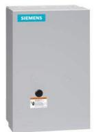
Non-reversing NEMA contactor, Size 3, Single phase full voltage, Contactor amp rating 90A, 3 wire (NO aux included), 110-120/220-240VAC 60Hz coil, Non-combination type, Enclosure NEMA type 1, Indoor general purpose use, Standard width enclosure
