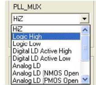
Figure 9 - Programming the PLL_MUX of the LMK03000C.
