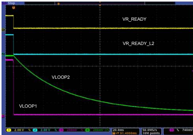
Figure 44: OCP on Loop #1 shuts down both loops
