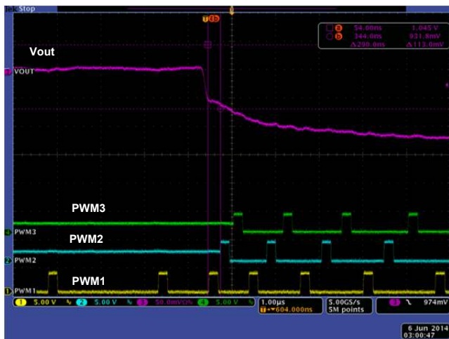
Figure 39: Phase Add 1\Phi \rightarrow 3\Phi
