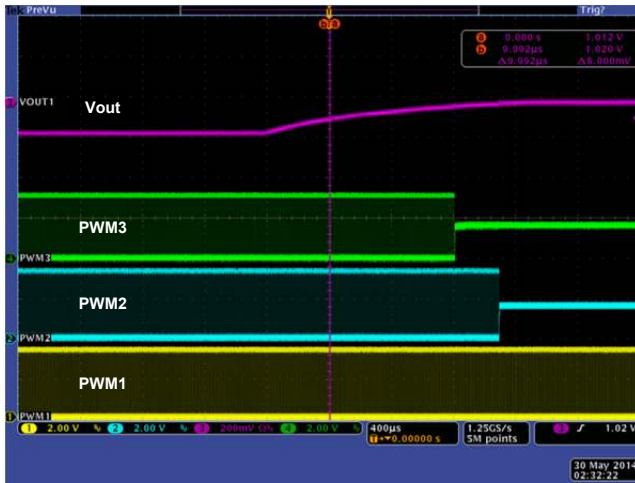
Figure 38: Phase Shed 3\Phi \rightarrow 1\Phi
