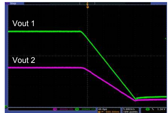
Figure 20: MPoL Tracking Shutdown
