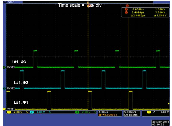
Figure 21: 3-phase PWM interleaved operation
