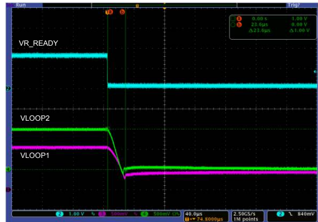
Figure 43: OVP - MOSFET released when output<0.5V
