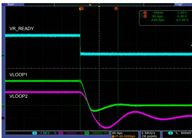
Figure 42: OVP - MOSFET latched on
