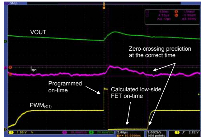
Figure 41: PS2 Active Diode Emulation Mode
