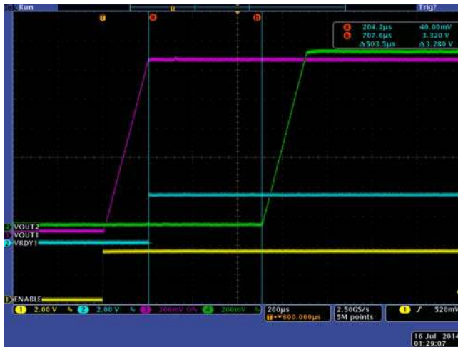
Figure 16: Loop 2 starts when Loop 1 VRRDY = high with 0.5ms delay between the loops
