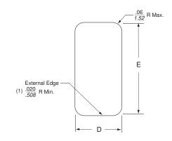
Note: The external edges (installation side) on the "D" sides of the cutout should have a minimum .020" radius. For optimal retention against extraction, the corresponding inner edge should be sharp, without paint or coatings. Edge coatings, including anodization are also discouraged for good shield contact.
