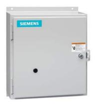
Mechanically held lighting contactor, Contactor amp rating 20Amp 0NC  $\_$  8NO poles, 208-240V 50/60HZ coil, Non-combination type, Enclosure NEMA type 12, Dust/drip proof for indoors
