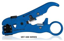
The UST Series creates a two step strip on a multitude of cables (and the UST-175 provides a three step strip). These tools include a Velcro strip for folding back the braided shield of the cable. Cartridge blades are interchangeable and capable of making over 5,000 cuts.
