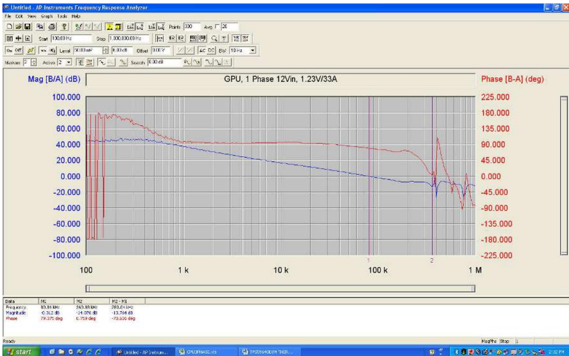
Figure 71. GPU Bode Plot at 12Vin, 1.23 V/33 A
