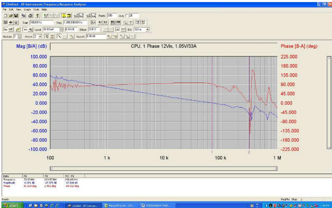
Figure 57. CPU1 Bode Plot at 12Vin, 1.05 V/33 A
