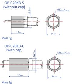
Note: When attaching, make sure that the side without a bearing chamfer is the impact surface.
