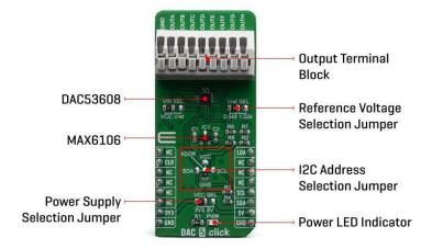
The DAC 5 click has a high precision voltage reference included onboard. For that purpose, MAX6106 is used, a 2.048V voltage reference IC, from Maxim Integrated. This little SOT23 device is stable with capacitive loads, and no output capacitor is required. It has regulations for both sink and source and is very accurate. This gives DAC 5 click good flexibility for use in various applications.
