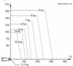
The KR 10 R900-2 is designed for a rated payload of 5 kg in order to optimize the dynamic performance of the robot. With reduced load center distances, higher loads up to the maximum payload may be used. The specific load case must be verified using KUKA.Load. For further consultation, please contact KUKA Support.
