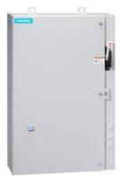
Non-reversing motor starter Size 3 Three phase full voltage Solid-state overload relay OLRelay amp range 25-100A 24VAC 50-60HZ coil Combination type 125Amp circuit breaker Enclosure NEMA type 4/12 Water/dust tight for outdoors Standard width enclosure
