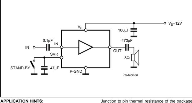
For 12V supply and  $8\Omega$  speaker application, its maximum power dissipation is about 1W.
