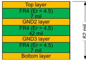
Figure 5-1. PCB Layer Stack-Up
