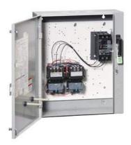
2-speed 3-phase motor starter Size 1 Two separate windings Constant or variable torque Solid-state overload relays Low SPD OLR range 0.75-3.4A High SPD OLR range 3-12A 110V 50HZ / 120V 60HZ coil Combination type 10Amp circuit breaker Enclosure NEMA type 4/12 Water/dust tight for outdoors
