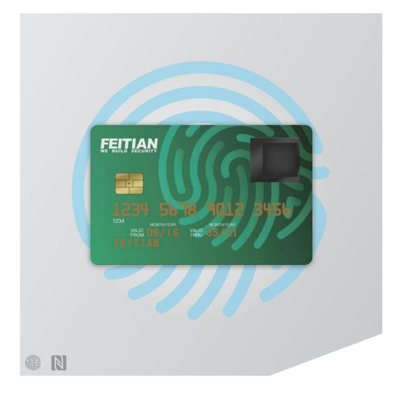
Biometric on card, with the flexible biometric sensor and the strong matching chip embedded.
