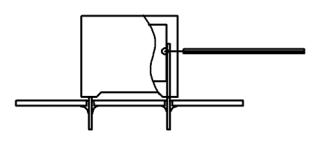
Temperature monitored inside the capacitor.
