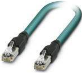
Patch cable, CAT5e, 4-pair, shielded, line, assembled at both ends with straight RJ45/IP20 heads, length: 0.3 m
