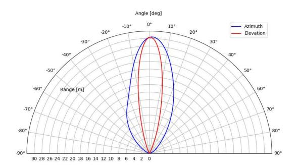
Note: In order to acquire the data for elevation, the sensor module has been turned by 90° clockwise with perspective from the sensor to the FoV.
