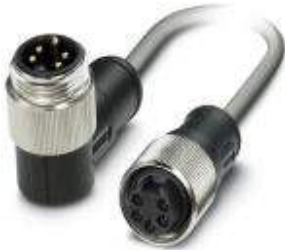
Bus system cable, DeviceNet, 5-position, PUR halogen-free, Gray RAL 7001, Plug angled 7/8"-16UNF, on Socket straight 7/8"-16UNF, Cable length: 20 m
