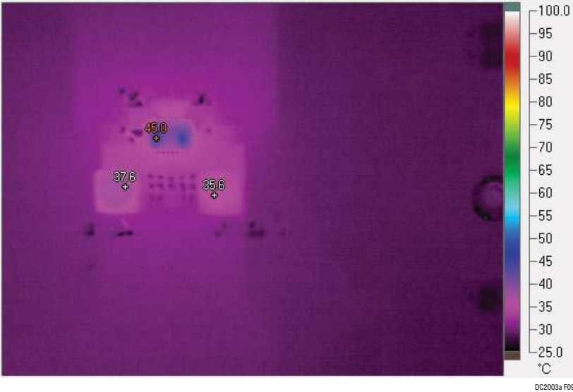
Figure 9. Thermal Performance at V_{IN} = 12V , V_{OUT1} = 3.3V , I_{OUT1} = 1A , V_{OUT2} = 5V , I_{OUT2} = 1A , F_{sw} = 1MHz , No Airflow
