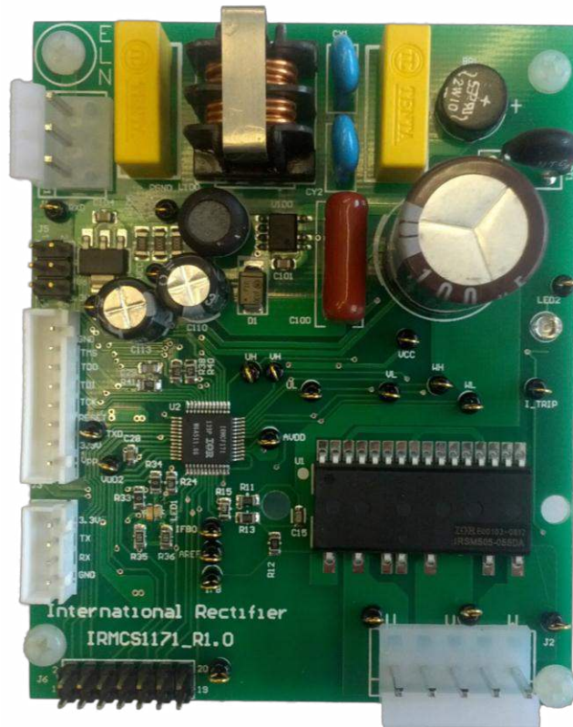
Figure 4: Reference design board featuring the \mu IPM™-DIP module and the iMotion™ IRMCF171 digital control IC
