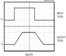
$\begin{aligned} &V_{CC}=\pm 2.5V\\ &R_L=100k\Omega,\ C_L=15pF\\ &A_V=1V/V \end{aligned}$
