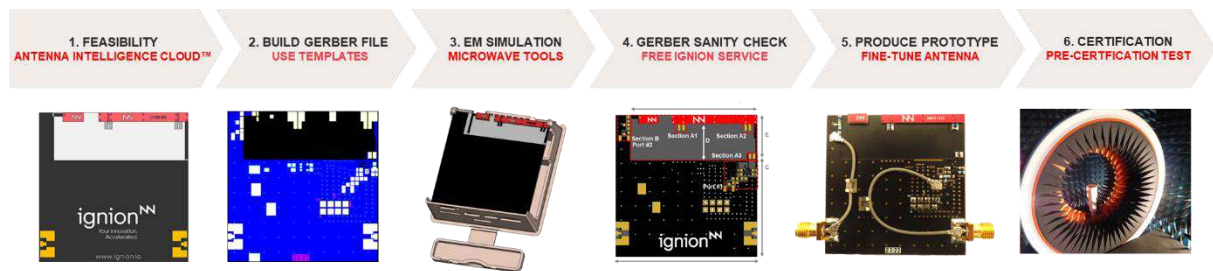
Figure 12 – Virtual Antenna® design journey for a successful IoT solution.
