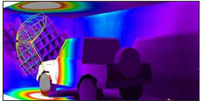
Garage : false color with light distribution
