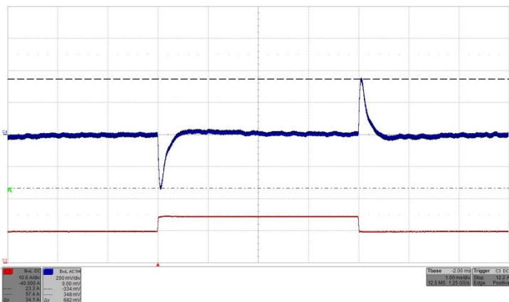
Fig. 53: Output voltage response to load current step change 50% - 75%-50% (9.5A–14.25A–9.5A) with di/dt = 1A/\mu s at V_{in} = 24V . Top trace (C4): Output voltage (200 mV/div.). Bottom trace (C3): Load current (10A/div.). Time: 1ms/div.
