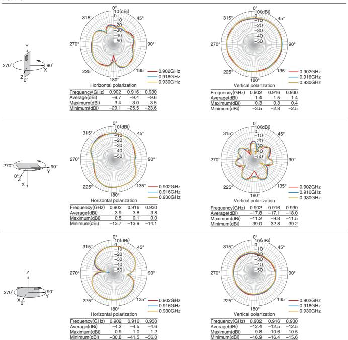
• Tested antenna has been soldered. Evaluation board size is 100x20x1mm.
