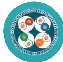
Ethernet, flexible, CAT5e [94B]
