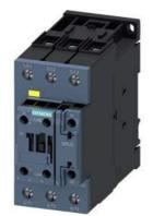
power contactor, AC-3e/AC-3, 80 A, 37 kW / 400 V, 3-pole, 83-150 V AC/DC, 50/60 Hz, with integrated varistor, auxiliary contacts: 1 NC, screw terminal, size: S2, F-PLC-IN
