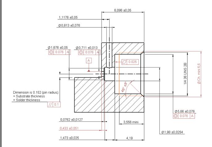
To obtain correct concentricity and dimensions on the receptacle piercing, we recommend to use RADIALL special tools:
