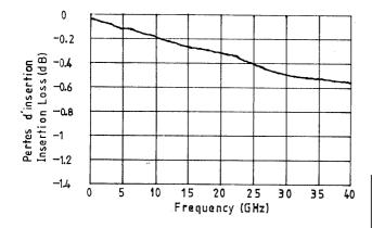
Insertion loss measurements in coaxial circuit with glass bead
