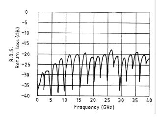
Typical return loss of a connector pair with two glass beads joined by 1 inchmicrostrip
