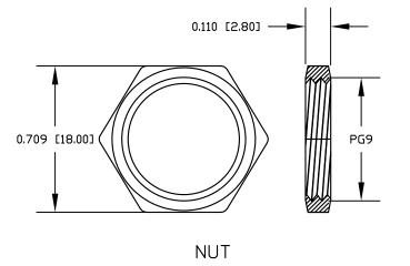
NOTE: MATERIAL HDUSING: PBT UL94V-0, BLACK CONTACT: **BRASS** NUT: **BRASS** SHELL: **BRASS** D-RING: EPDM, BLACK **FINISH** CONTACT: GOLD PLATED, 10 µ" Min. UNDER PLATE: NICKEL NICKEL PLATED NUT: SHELL: NICKEL PLATED **ELECTRICAL** RATED CURRENT: 4A RATED VOLTAGE: 250V INSULATION RESISTANCE: 100ΜΩ ΜΙΝ CONTACT RESISTANCE:  $10m\Omega$  MAX IP67/68
