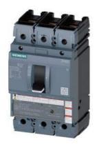
circuit breaker 3VA5 UL frame 250 breaking capacity class H 65kA @ 480 V 3-pole, line protection TM230, FTAM, In=250A overload protection Ir=250A fixed short-circuit protection Ii=5...10 x In UL489 SB (naval), 50 deg. cel. nut keeper kit on both sides
