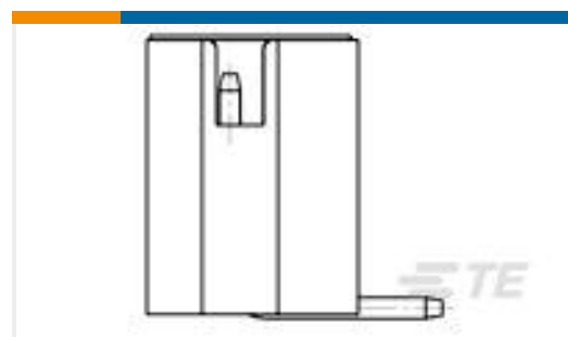
TE Part #1775317-7 HPI, 2.5MM PITCH, V/T, SMT TYPE, 7 POS
