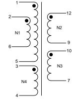
N1 denotes two windings connected in parallel. Terminals 1+2, 5+6 must be tied as solder bridging is allowed.
