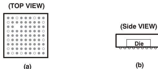
Figure 39. Views of Thermally-Enhanced GQE Package
