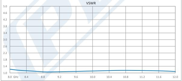
Click the following link (or enter part number in "SEARCH" on website) to obtain additional part information including price, inventory and certifications: Isolator with 20 dB Isolation from 8 GHz to 12 GHz, 10 Watts and SMA Male PE83IR1027
