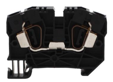
Feed-through terminal, Tension-spring connection, Mounting type: Mounting rail TS 35/7.5, Rated cross-section: 6 mm², Width: 8.1 mm, Colour: Black
