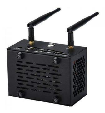
Honeycomb vents of the case reduce the heat generated by your device while it is performing neural network training or running machine vision programs. There are four anti-skid rubber pads on the bottom of the case to prevent skidding. We provide you with anti-static tweezers and screwdriver to help you to install easily; besides, we offer you three jumper caps to ensure the normal operation of reset and restart functions.
