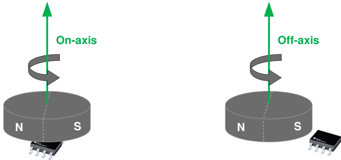
Figure 8-5. On-Axis vs. Off-Axis Angle Measurements
