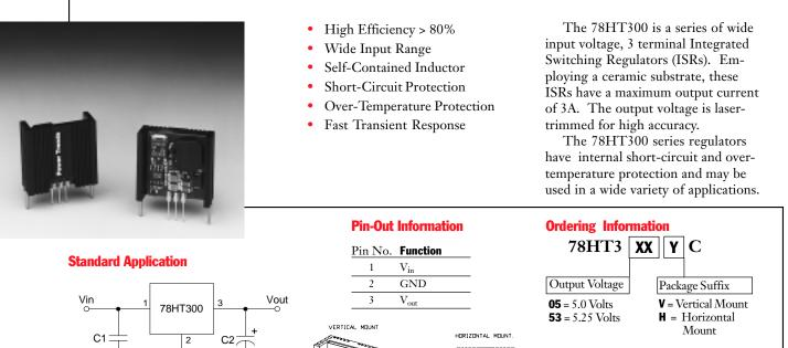
C1 = Optional 1µF ceramic C2 = Required 100µF electrolytic GND
