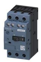
Special type Circuit breaker size S00 for motor protection CLASS 10 A-release 1.1...1.6 A N-release 21 A Screw terminal Standard switching capacity with transverse auxiliary switch 1 NO+1 NC Ambient temperature -50 °C 500 switching cycles
