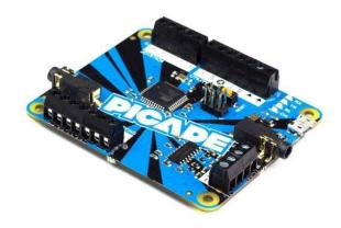
This is an Arduino-compatible board with integrated 3W stereo amplifier designed for use in arcade projects (like our Picade).
