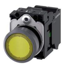
Illuminated pushbutton, 22 mm, round, plastic with metal front ring, yellow, pushbutton, flat, momentary contact type, with holder, 1 NO, LED module with integrated LED 24 V AC/DC, Spring-type terminal
