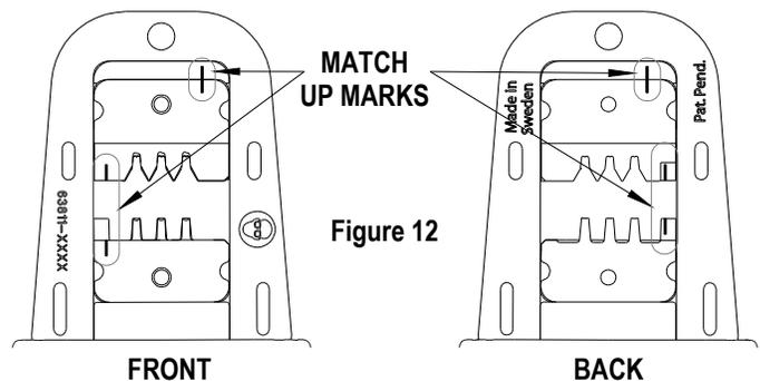
3. Flip the upper tooling to the opposite side and replace the M3 BHCS. Make sure the small markings on the front and back of the hand tool frame match up and are on the outside of the hand tool frame. See Figure 8 and 9.
